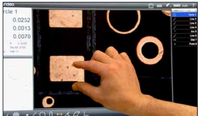
Feature measurements can be performed using common touchscreen operations such as pan and pinch zoom. Or use conventional mouse operations like point and click.
