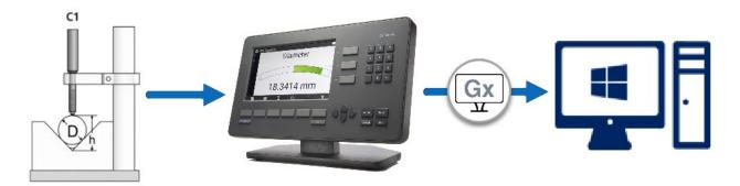
To send data from an Gx200 to an instance of the GxLink software, the Gx200 must have GxLink enabled in setup and the readout connected to a network.
